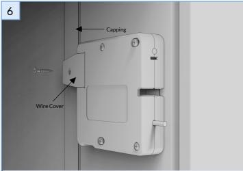
Fit the aluminium extrusion capping if appropriate. Press the wire cover into place and fasten with 25mm wood screw. This locker is now complete. Repeat process for all lockers
