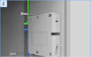
Align the lock with the predrilled holes in the locker wall. Insert the 2 lock screws through the slotted bosses and fasten. These slots will allow you to fine tune the locks positioning later. CONNECT THE CABLES NOW
