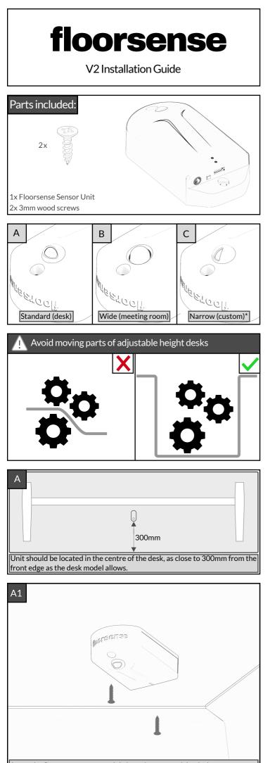
Screw the floorsense sensor module in to the centre of the desk.
