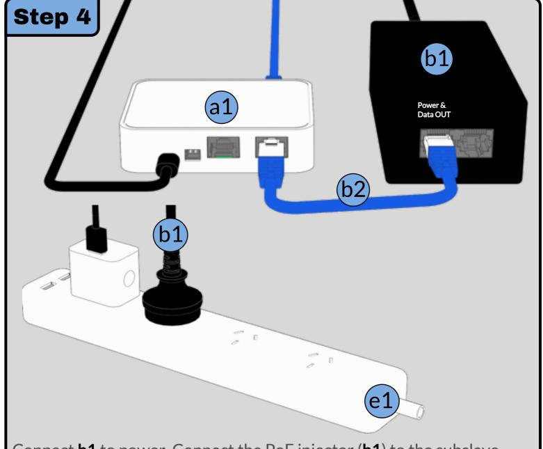
Connect **b1** to power. Connect the PoE injector (**b1**) to the subslave controllers (**a1**) CAN board via RJ45 Cable. Ensure it is plugged in to **Power & Data OUT** port on **b1**.
