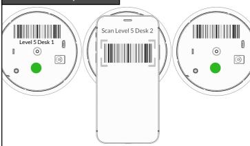
The camera will open. Point the camera at the barcode on the bottom of the module. A coloured line will flash across the barcode (on the phone screen) and the corresponding serial number will automatically write out to the selected cell in the spreadsheet. Repeat steps 3 and 4 until all the desks on that level have been mapped.
