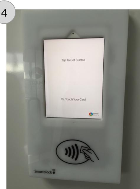
If the Kiosk App shows WIFI not connected it may have a problem reconnecting to the WIFI even though the controller is working properly. To rejoin the WIFI first stop the Smartalock Kiosk app from running by pressing the home button.
