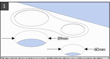
If the desk does not have a pre-drilled hole then you will need to do this with both a 3.5 (89mm) inch and 60mm holesaw. See accompanying drawing for detail.
