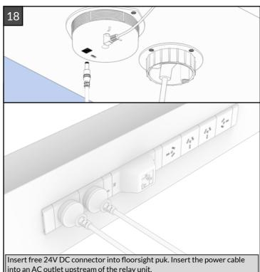
into an AC outlet upstream of the relay unit.
