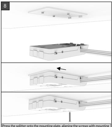
Press the splitter onto the mounting plate, aligning the screws with mounting holes. Slide the unit until it clips firmly into position. (Optional: Lock in place with 4x25mm wood screw).
