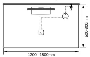
The floorsight module requires an 89mm (3.5inch) hole in the desk. The module is pressed in to place and provided power via a 20 volt AC-DC power adapter connected to below-desk mains power output. The floorsight module is then connected to the below-desk floorsense module via a 3.5mm stereo cable. See floorsen.se/support for more information.
