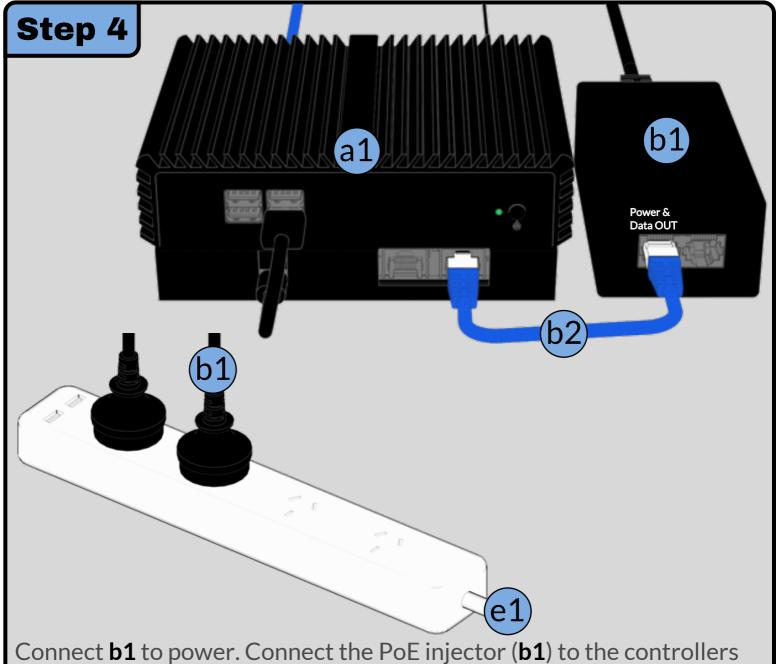
Connect **b1** to power. Connect the PoE injector (**b1**) to the controllers (**a1**) CAN board via RJ45 Cable. Ensure it is plugged in to **Power & Data OUT** port on **b1**.
